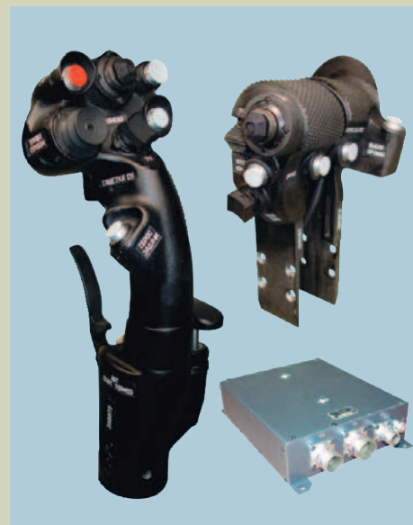
Set of aircraft control stick and throttle control knob KNOPKA
